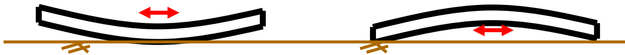
Figure 2.2. Locations of critical stresses due to slab curling and warping (Wells et al. 2005).
