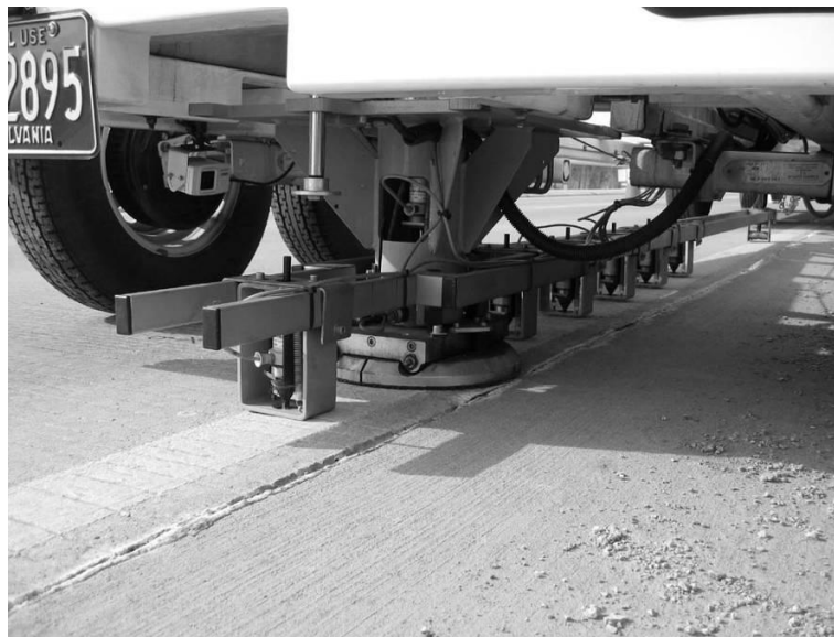
Figure 7.1. Falling weight deflectometer (FWD) load plate and sensor configuration.
