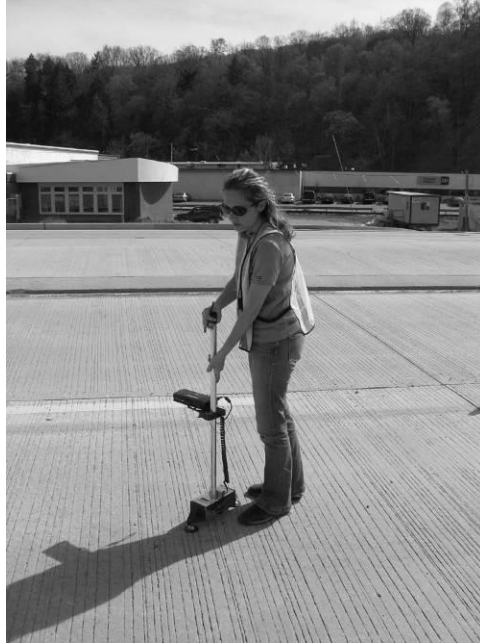
Figure 6.41. Surface profile measurements using the Dipstick™.
